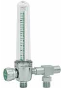
Flowmeter with Power Take Off Connector NFPA 99 Color coding, Inlet: 1/8" NPT(F), Outlet: DISS
